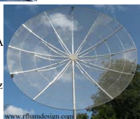
Dish A_e \doteq 0.55A D = 2.4\text{m}, A_e = 2.5\text{m}^2 @ 400\text{MHz}
