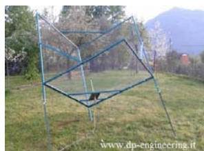
3-D Corner Reflector A_e = 5\lambda^2 = 2.5\text{m}^2 @ 400\text{MHz}
