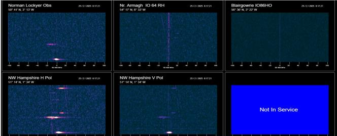
Bright horizontal lines are head echoes from meteors as they burn up and decelerate.
