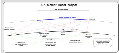
Data from up to six receivers are streamed to the project server where it is recorded for later analysis.
