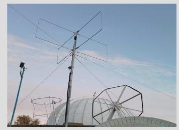
A transmitter located at the Sherwood Observatory near Mansfield illuminates this region above the UK and a network of receivers monitor and record the echoes.
